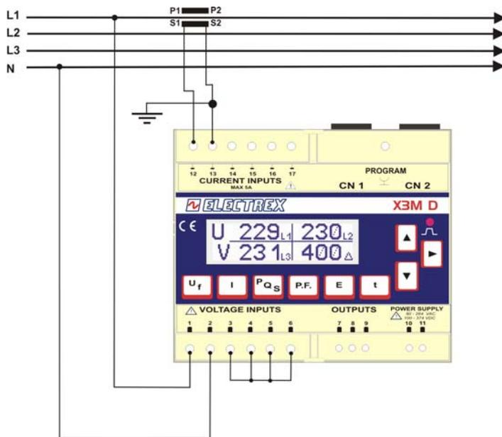
Low Voltage 1 CT (symmetrical and balanced load)
