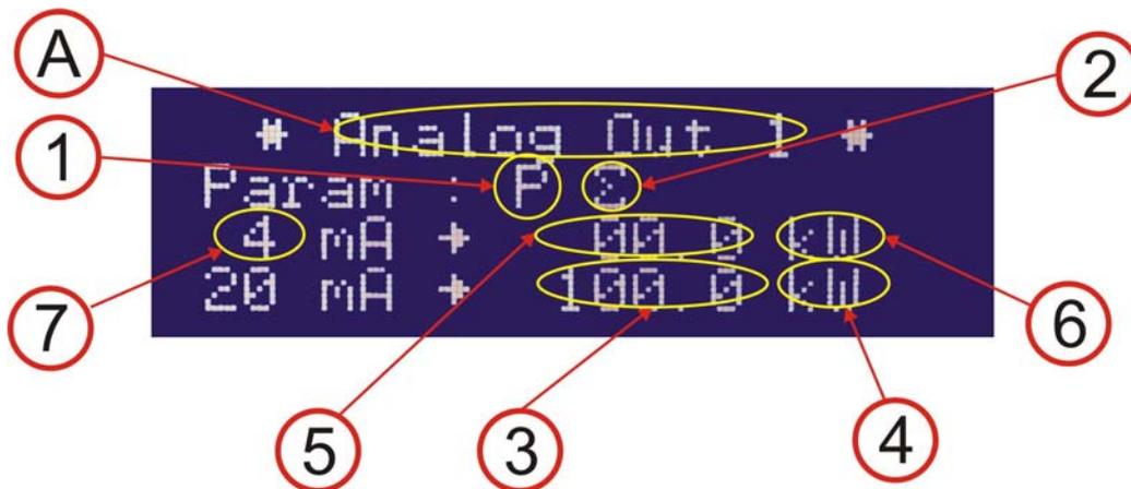
(A) Output identification: **A.o.1** = analog output 1.
