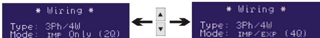
The first selection sets the type of electrical system and the type of wiring used:
