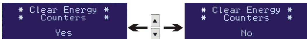
It is also possible to exit the procedure, at any time without resetting, by pressing the PROGRAM button.
