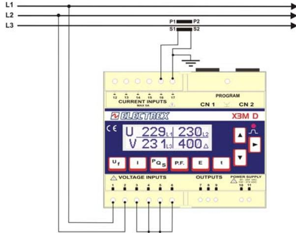
Low Voltage 1 CT (symmetrical and balanced load)
