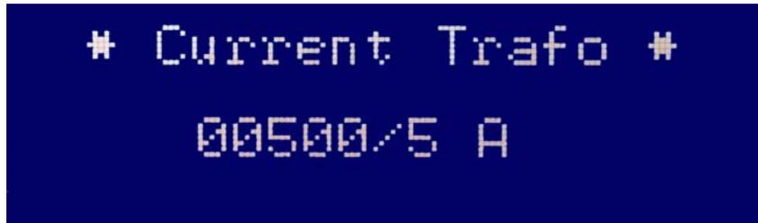
Ensure to enter the CT rated primary and secondary values as indicated on the CT label. When using 2 or 3 current transformers ensure that all the current transformers have the same ratings. The instrument is set by default to [**00005/5**].
