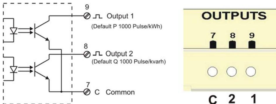
In order to calculate the energy value of each pulse the following formula must be considered.
