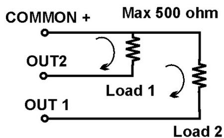
NB. The outputs are self powered; do not use external power supply.
