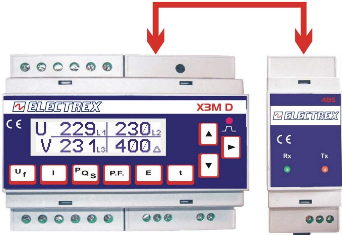
CN1 connector: suitable for the RS485 or RS232 optional modules
